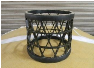
Fig 6. Fabricated Gridded Cylindrical Lattice Structure
